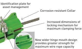
provides greater strength for maximum wire rope capacity
