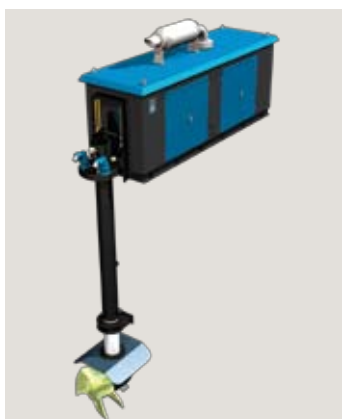
Deck mounted thruster units placed on deck, with containerised prime mover
